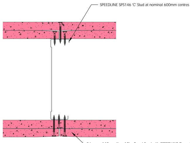
2 layers of 15mm Knauf Fire Panel fixed with SPEEDLINE Drywall Screws at 300mm centres (200mm centres at external angles). Ref to table for fixing length.
